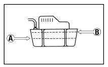
NOTE: If the water level rises above level (B), COOL operation will automatically shut off. Contact your MovinCool reseller for repair.
